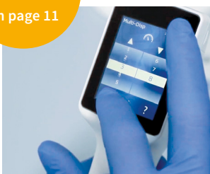
Setting the aspiration and dispensing speed
